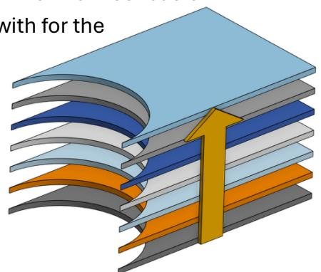
One can also extrude with a **draft**, which scales (shrinks or magnifies) the cross-sections proportionally throughout the distance of the extrusion. In this case, each cross-section is geometrically similar, but not congruent, to the original. The amount of scaling is controlled by the **draft** – the angle at which the surface is bent inward or outward from the base.
