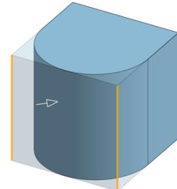
When more complex forms are tackled, there will be numerous sequences that get the job done. Sometimes, a student may build up a shape in steps with the extrude “Add” option or make a shape and then “Remove” unwanted regions. For example, for the Lego-style brick activity, we removed the inner region, but could have instead started with a relatively flat top surface and then added the four walls.
