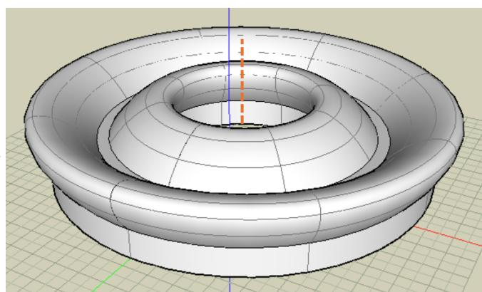
If the axis of rotation does not intersect the sketch, as in the example above, the resulting shape will have a hole. The axis cannot be internal to the shape; it can only be an external edge or non-intersecting line. Internal axes lead to self-intersecting shapes and OnShape will not generate a figure. Rotations can be less than 360° like a cake with a missing wedge.
