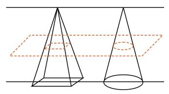
pairs in each plane, then the two solids have the same volume. At right is an image that is part of a classic derivation of the formula for the volume of a cylinder (the pyramid is already known to be 1/3(area of Base)(Height) which leads to the same formula for cylinders). The proportions of the shapes are chosen so that at each level, the square cross section and circle cross section have the same area, so the two solids have the same volume.
