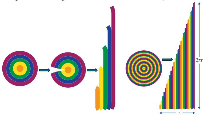
width), then those open up into a triangle made of an infinite number of segments. The triangle has a base of r and a height equal to the outermost disk's circumference, or  $2\pi r$ . Finding the area of the triangle yields  $A = \frac{1}{2}(r)(2\pi r) = \pi r^2$ , which is therefore the area of the circle as well. This dissection is Cavalieri-like in the sense that we are pairing equal lengths in the circle and triangle as we sweep radius values from 0 to r.
