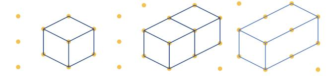
Note that when drawing multiple cubes, it is easiest to start with the one closest to the viewer (you) and then add ones that are partly obscured by that first cube. It is easier to picture which edges of the cube should be omitted that way.
