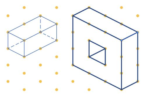
Isometric drawings may be ambiguous. We don't know if the two shapes pictured here are the same or not, because we can't see if the left image has a missing corner hidden in the back (imagine rotating the righthand figure up and over).
